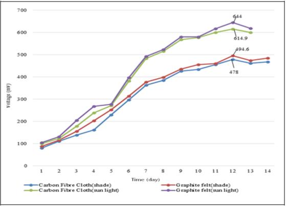
Figure 7: variation of average daily voltage with electrode material
