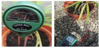
Figure 4: Three-Way Meter and Digital multimeter
